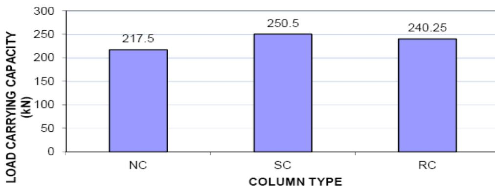
**Figure 4.3 Comparison of load carrying capacity of NC, SC and RC (Specimen 'B')**
