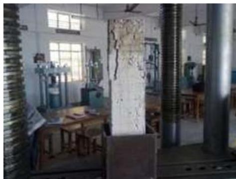
**Figure 4.1 Failure pattern of normal column**
