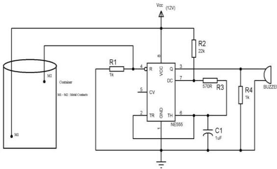
Fig 2: Digital Water level Indicators
