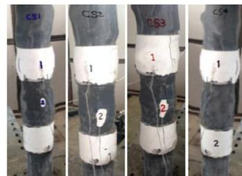
**Fig. 9.** Failure modes for CFT PVC columns with plain socket
