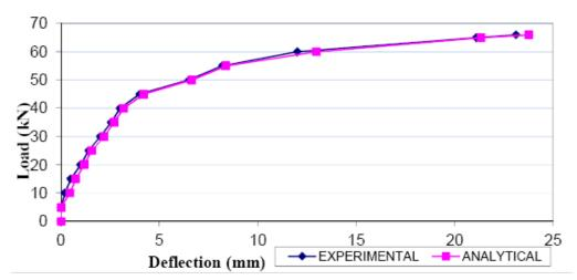
Figure 5.5 Comparison of analytical and experimental load deflection curve of bottom half portion wrapped flexure strengthened beam
