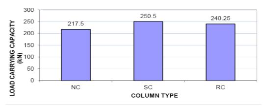
Figure 4.3 Comparison of load carrying capacity of NC, SC and RC (Specimen 'B')
