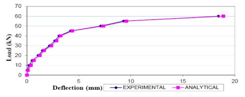
Figure 5.3 Comparison of analytical and experimental load deflection curve of flexure beam
