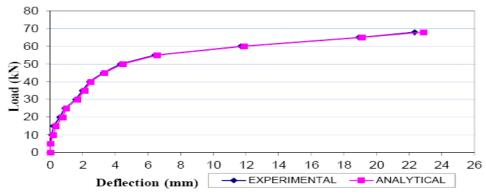
Figure 5.4 Comparison of analytical and experimental load deflection curve of full portion wrapped flexure strengthened beam
