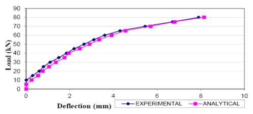
Figure 5.2 Comparison of analytical and experimental load deflection curve of normal strengthened beam
