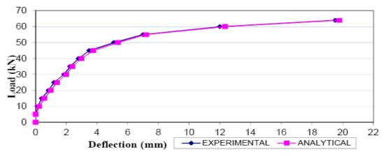
Figure 5.6 Comparison of analytical and experimental load deflection curve of middle one third portion wrapped flexure strengthened beam
