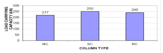
Figure 4.2 Comparison of load carrying capacity of NC, SC and RC (Specimen 'A')
