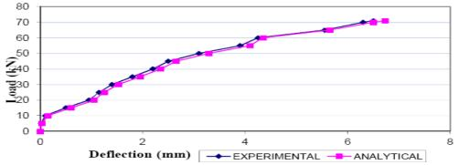
Figure 5.1 Comparison of analytical and experimental load deflection curve of normal beam
