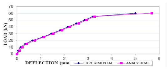
Figure 5.7 Comparison of analytical and experimental load deflection curve of shear beam
