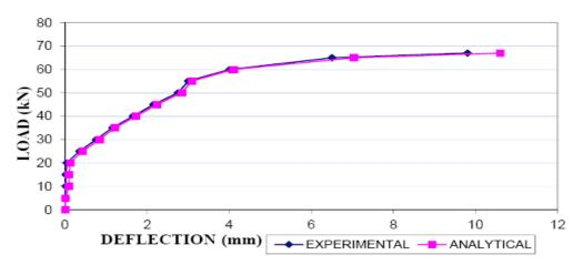
Figure 5.8 Comparison of analytical and experimental load deflection curve of shear strengthened beam
