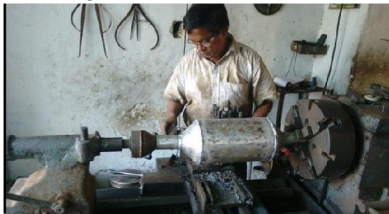
Fig7: Fabrication of catalytic convertor
