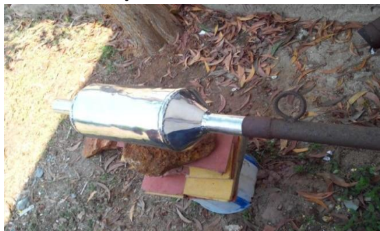
Fig8: Catalytic convertor fitted to engine exhaust
