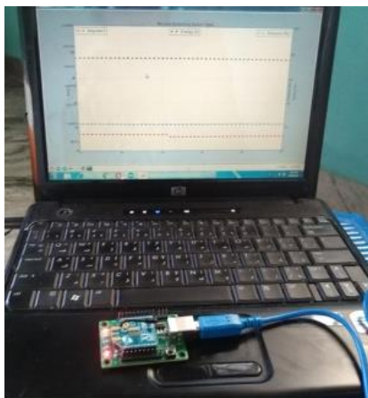
Fig. 8: Receiving Node connected to a graphical interface.
