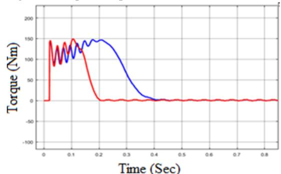
Fig. 14. Torque comparison of 11-level PI and FIS
