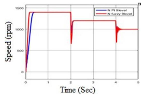
Fig. 10. Speed variation of 9-level PI and FIS
