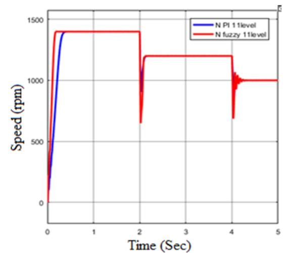
Fig. 11. Speed variation of 11-level PI and FIS
