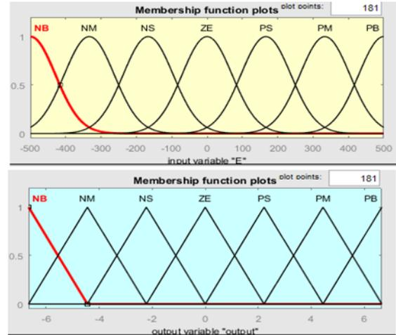
Fig. 4. Input and output variable membership functions
