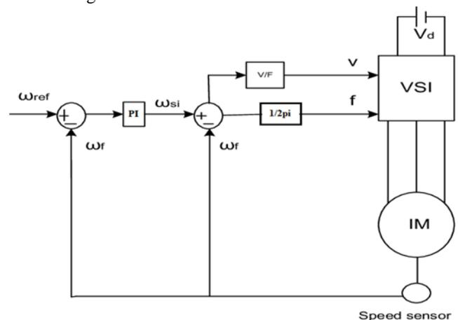
Fig. 1. 2-stage structure of induction motor operation
