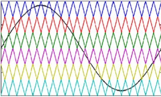
Fig. 3. Level shifted PWM technique for 7-level diode clamped inverter
