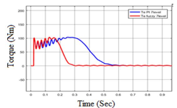
Fig. 12. Torque comparison of 7-level PI and FIS
