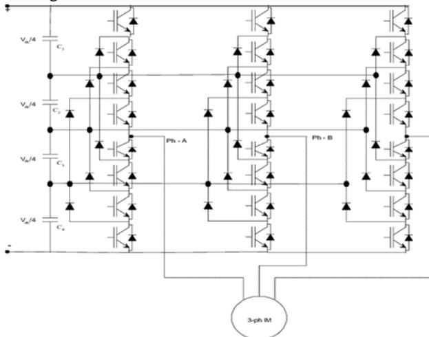
Fig. 2. Seven level diode clamped inverter topology with induction motor
