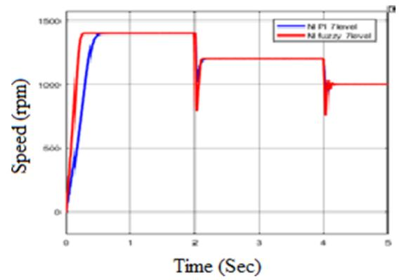
Fig. 9. Speed variation of 7-level PI and FIS
