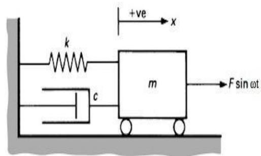
Fig 1: Damped Harmonic Oscillator
