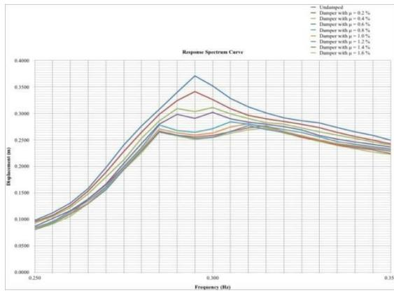
Fig 5: Response Spectrum Analysis curve for building with damper for varying mass ratios
