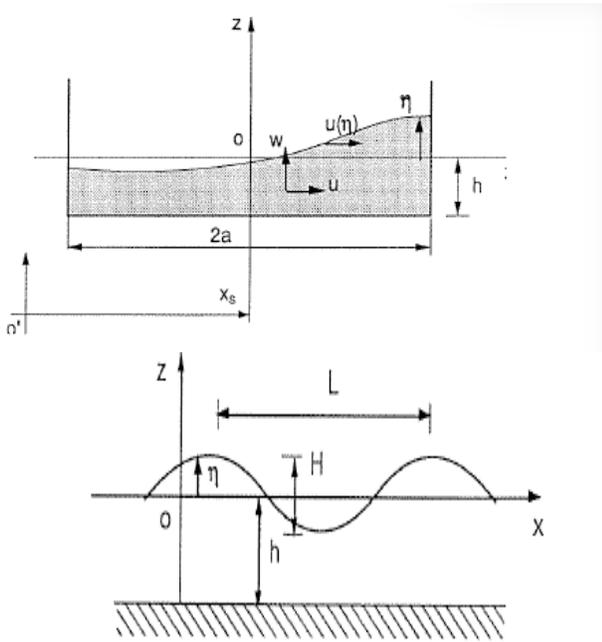
Fig 2: Schematic Diagram Showing Wave
