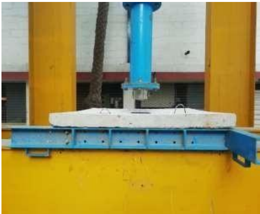
Fig. 2. Test Setup of Slab
