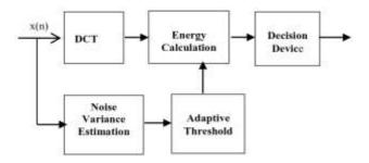
Fig.1: Block diagram of Enhanced Compression Based Spectrum Sensing.
