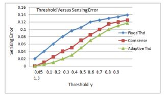
Fig.5b: Threshold Versus Spectrum sensing error for (SNR=3dB).
