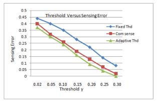
Fig.5a: Threshold Versus Spectrum sensing error for (SNR= 3dB).
