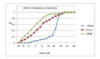
Fig.2: SNR Versus Probability of detection for low and high SNR regions.
