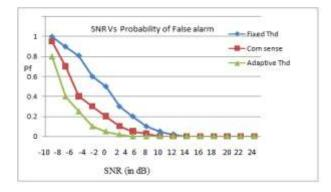
Fig.3: SNR versus Probability of False Alarm P<sub>f</sub> for low and high SNR regions.
