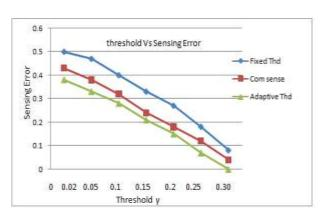
Fig.4a: Threshold versus spectrum sensing error for (SNR= -3dB)
